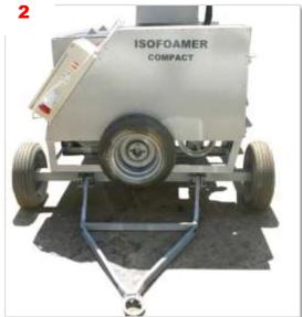
The ISOFOAMER COMPACT unit produces homogeneous cement/water or cement/sand/water in all densities requested for the final lightweight foam cellular concrete and pump it to the required destination.
