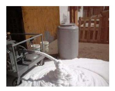
Isofoamer Infinity is a continuous foam generator specially designed for the production of lightweight foam concrete for densities varying from 300 up to 1200 Kilograms per cubic meter.
